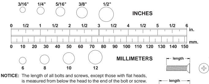
Is measured from below the head to the end of the bolt of screw. Flat head bolts and screws are measured from the top of the head to the end of the bolt or screw.
